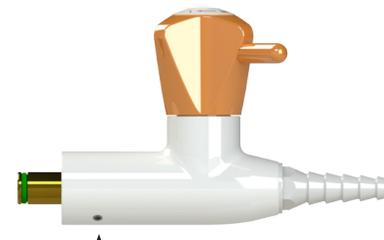
Tighten the two pointed screws, with a Hexagon key 2 mm, after mounting in the valve. Max. 1 lb-ft.
